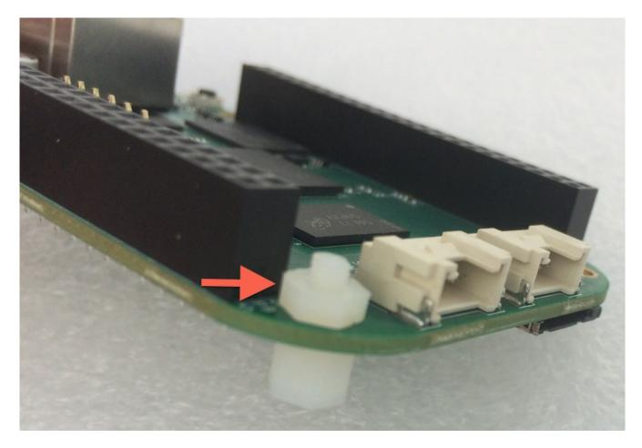
Attach plastic spacers to the BeagleBone at the four mounting holes in the corners. Tighten only fingertight. Do not use the metal screws on the BeagleBone as they may short the circuit board traces.
