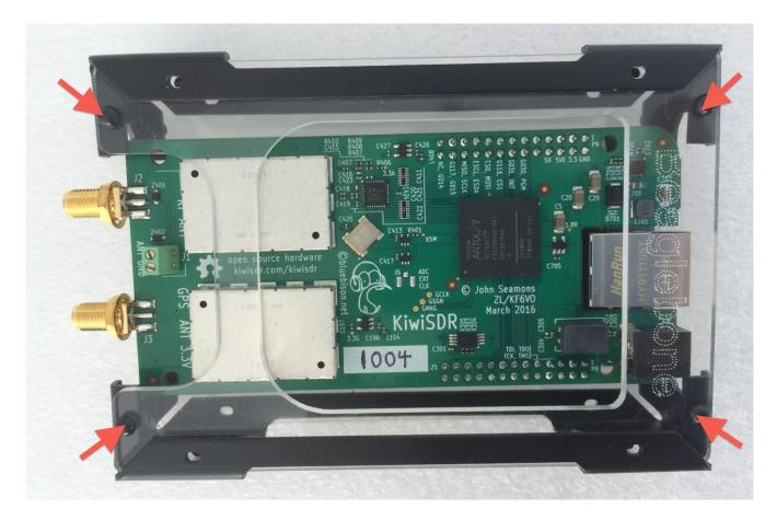
Insert plastic rivets at the four locations shown. This completes the enclosure assembly.
