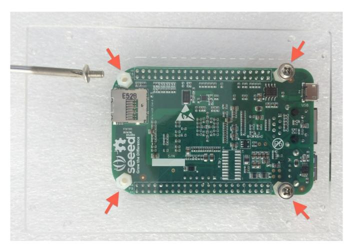
Attach BeagleBone to the bottom plastic plate with four metal screws using a Phillips screwdriver. Observe the etched markings on the plastic for correct orientation. An outline drawing of a micro-SD card and USB connector is etched into the plate. The Beagle Ethernet connector should be at the outside edge of the plate.
