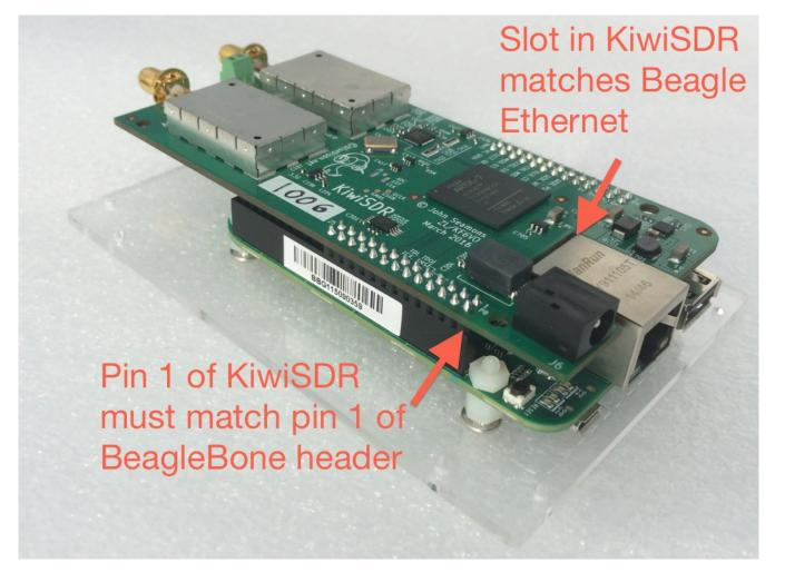
Attach KiwiSDR to BeagleBone. Be extremely careful to align the KiwiSDR pins into the correct header sockets of the Beagle. The cutout in the KiwiSDR board should wrap around the Beagle Ethernet connector with equal clearance on all sides. Push the KiwiSDR all the way down onto the Beagle headers as far as it will go. This allows enough clearance for the top plastic plate installed later on.
