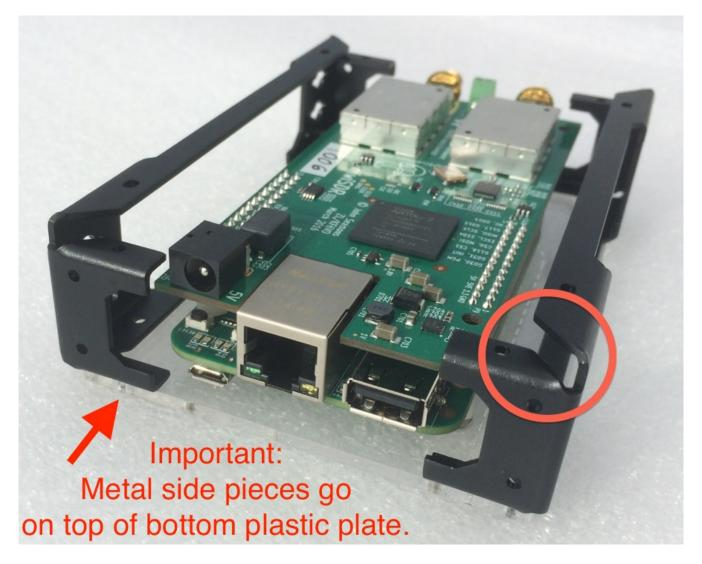
Position the metal side pieces. Note that the top of the side pieces have a slot for the insertion of the top plastic plate. Do not incorrectly exchange the left and right metal pieces so the slot ends up on the bottom.
