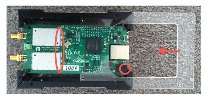
Note the orientation of the word "BeagleBone" etched into the top plastic plate. Slide the top plastic plate into the slots of the metal side pieces as shown. The plastic will just hit the KiwiSDR board at the circled locations. You should be able to lift the plastic plate very slightly and continue sliding it through the slots. This tight fit is why the KiwiSDR was pushed completely onto the Beagle headers in a previous step.
